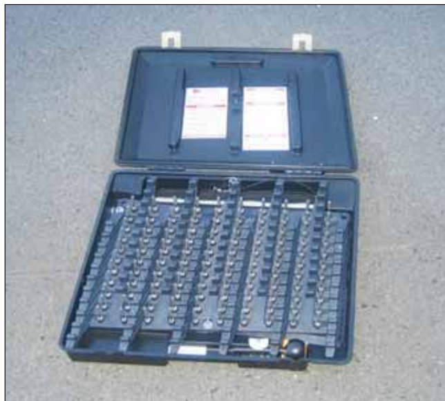
• The spikes come in a small, portable container (53cm x 45cm x 8cm) that can be slipped easily into any police vehicle.
