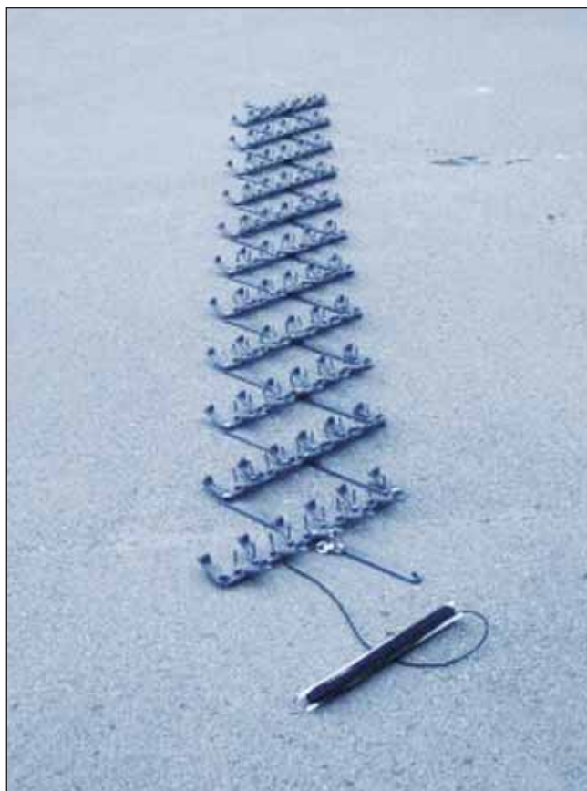
• The new lightweight, US-made Stinger road spikes stretch up to 10m and can penetrate any tyre, releasing air slowly to allow the driver to come to a slow and controlled stop.
